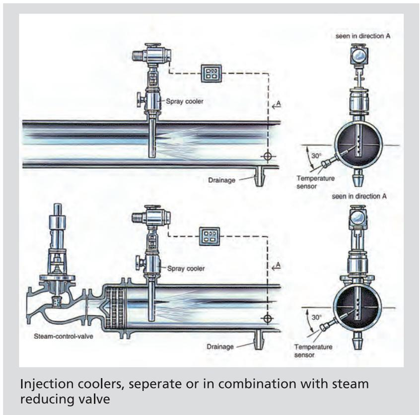
Injection coolers, separate or in combination with steam reducing valve
